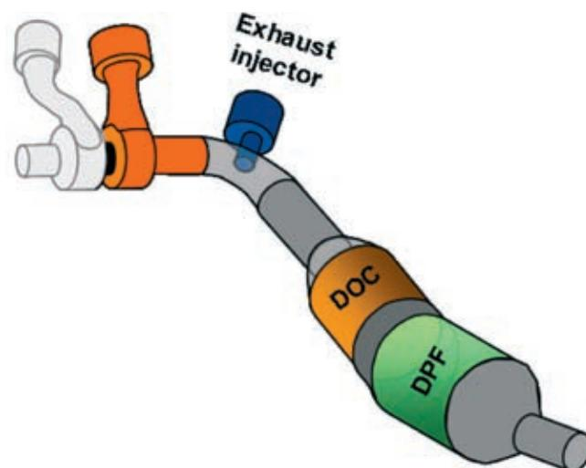
**Figure 12:** Euro 5 exhaust line layout
