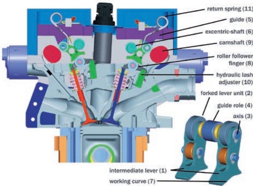
**Figure 2:** Modified cylinder head with "UniValve"
