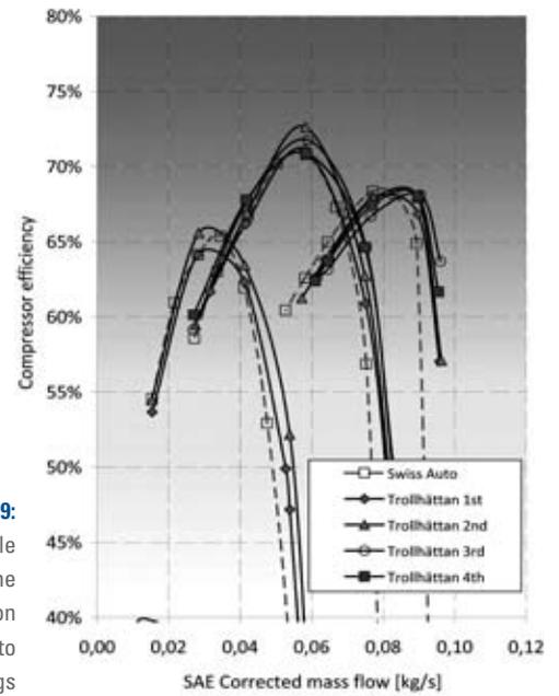
**Figure 9:** Good correlation example of repeated runs for the compressor efficiency on Saab/GM and Swissauto test rigs
