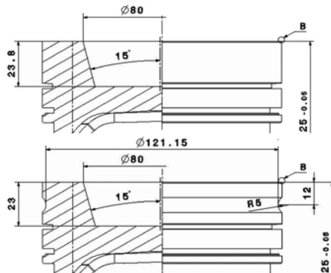
**Figure 8:** Geometry of the original piston (above) and the piston with increased volume of top land
