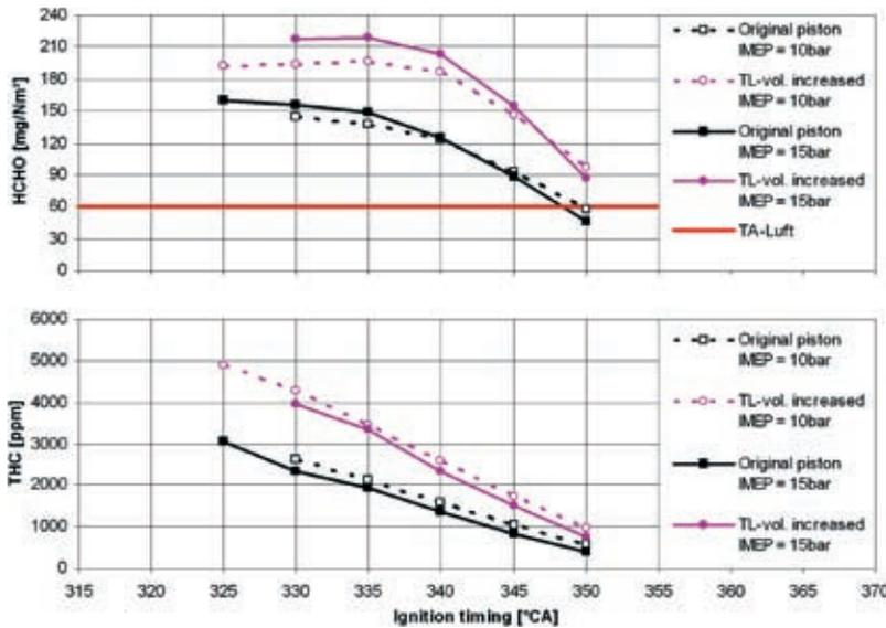
Figure 9: Formaldehyde (top) and hydrocarbon emissions (bottom) with enlarged top land volume
