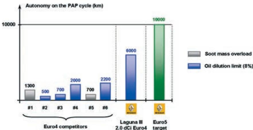
Figure 2: Comparison of the autonomy of Renault and competitors vehicles on the PAP cycle
