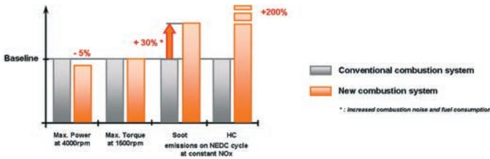
Figure 8: Comparison of the conventional and new combustion systems: power/torque at full load and emissions on the NEDC cycle
