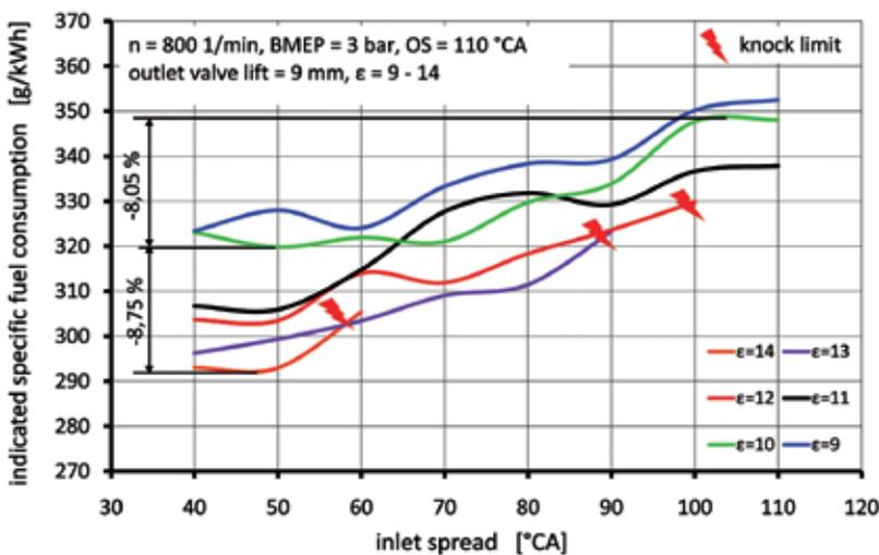
Figure 8: Indicated break specific fuel consumption over IS with variable compression ratio
