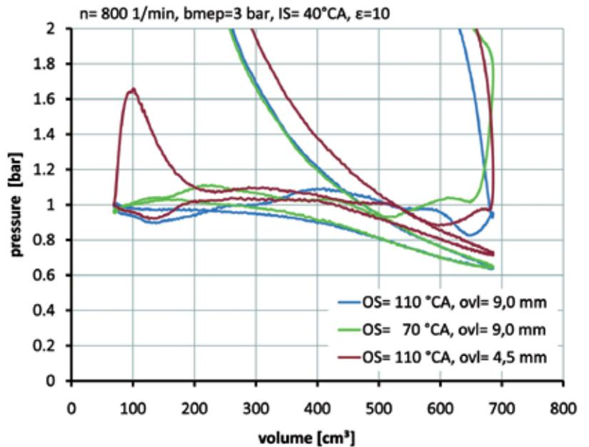
Figure 11: p-V diagram with variable exhaust valve
