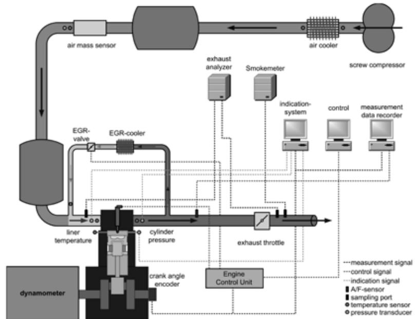
**Figure 2:** Schematic test bench setup
