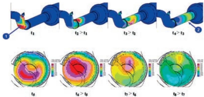
**Figure 14:** 3D CFD showing the evaporating and mixing processes as a function of time
