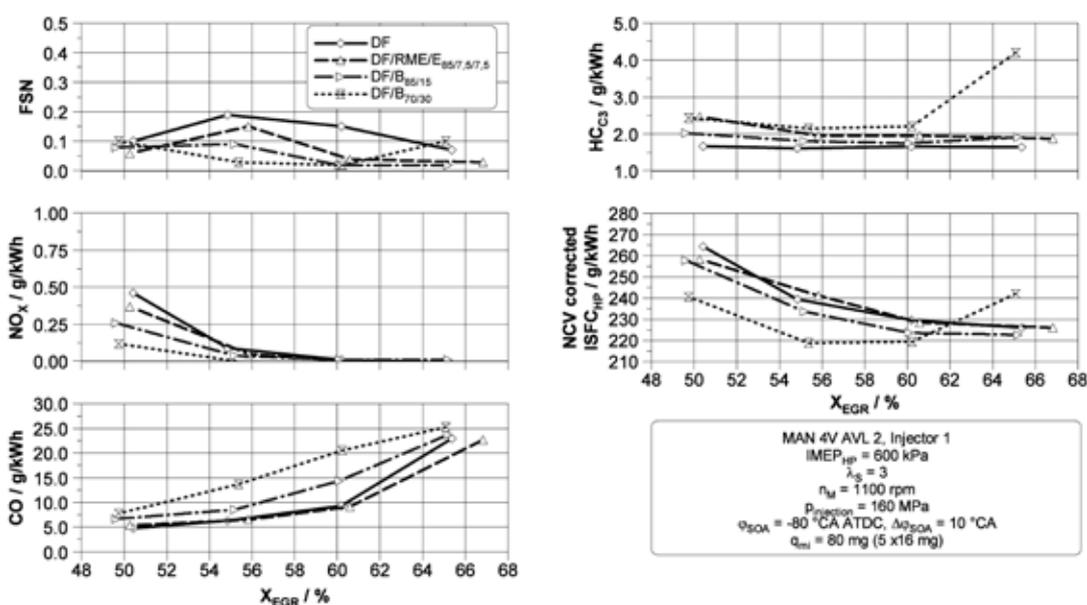
**Figure 5:** Emissions and specific fuel consumption, variation of EGR rate for different fuels at HDC, IMEP = 600 kPa
