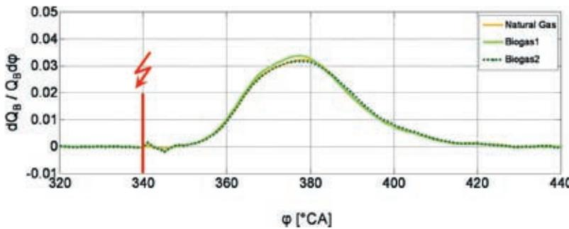
Figure 5: ROHR of the three fuel gases at IMEP = 10 bar and IP = 340° CA
