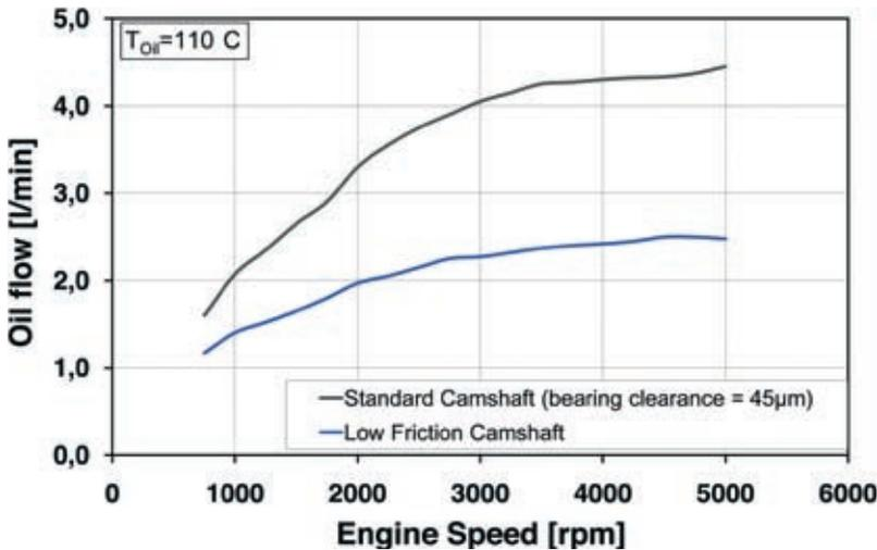
Figure 3: Reduced oil flow in the cylinder head through the use of an assembled camshaft with roller bearings
