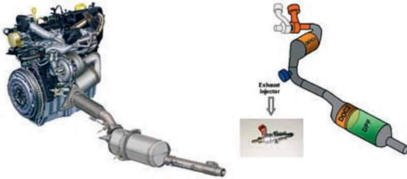
**Figure 3:** 1.5-dCi-Euro-4-DPF-engine (78 kW) equipped with the first generation of an exhaust fuel injection system
