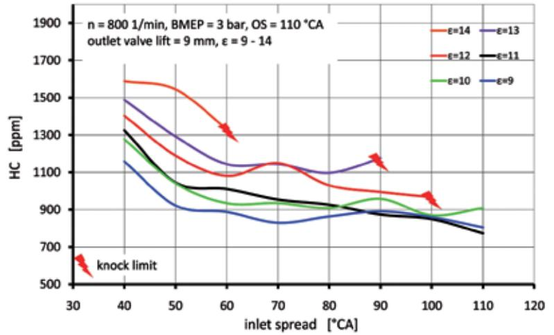
Figure 9: HC-emissions over IS with variable combustion ratio
