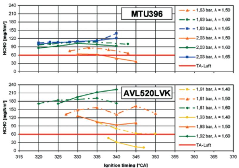
**Figure 3:** Emissions of formaldehyde in basic experiments for both research engines
