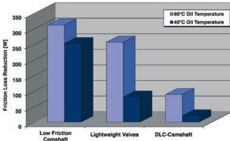
**Figure 1:** Average reduction in frictional loss resulting from optimisation measures in the valve train of a 16 V four cylinder engine
