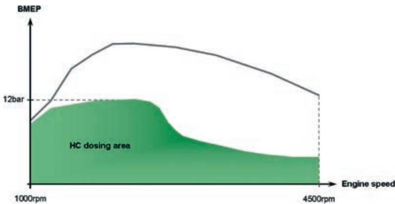
Figure 9: HC dosing area of the 1.5-dCi-Euro-4-engine
