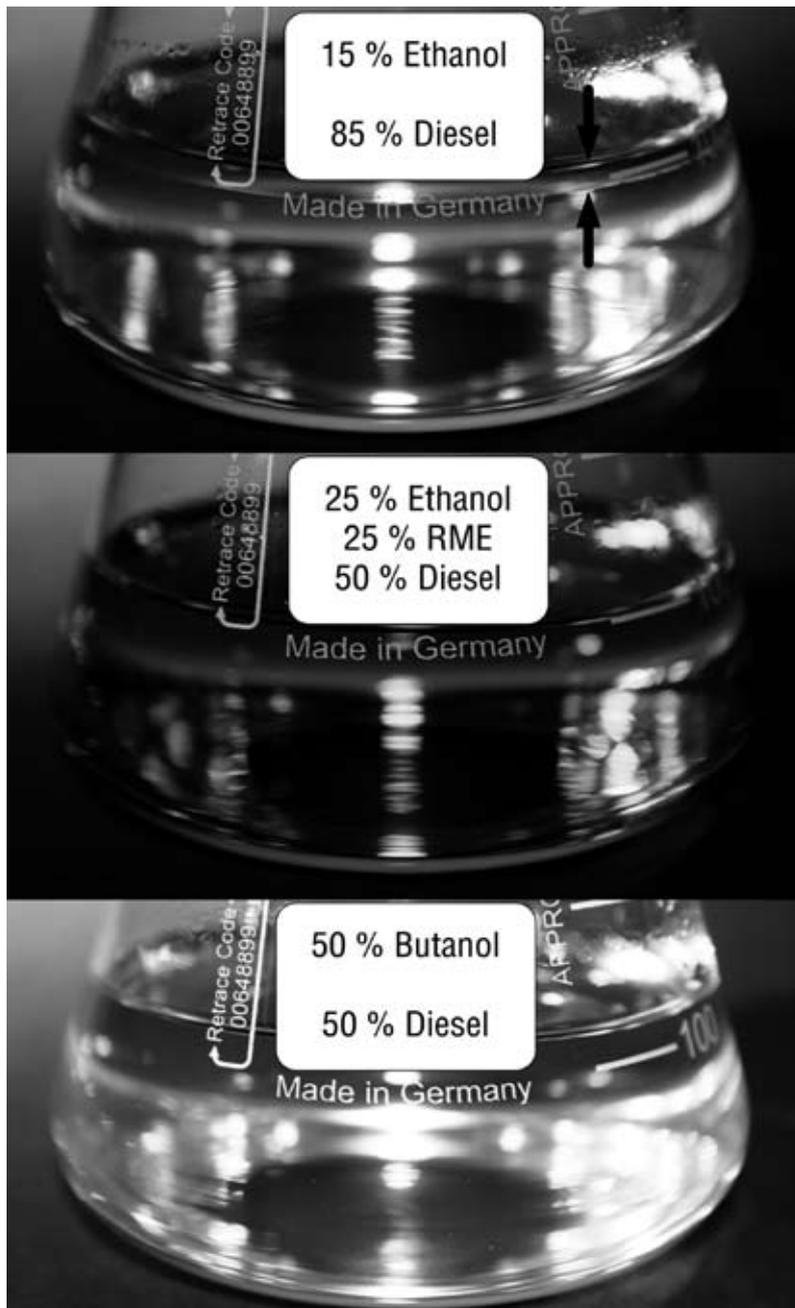
Figure 4: Study of miscibility of diesel with ethanol, RME and butanol
