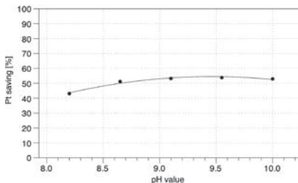
**Figure 5:** Platinum savings of channels prepared with precursors using biotemplates with regard to reference channels prepared without biotemplates (after aging at 850 °C for 24 hours in air)
