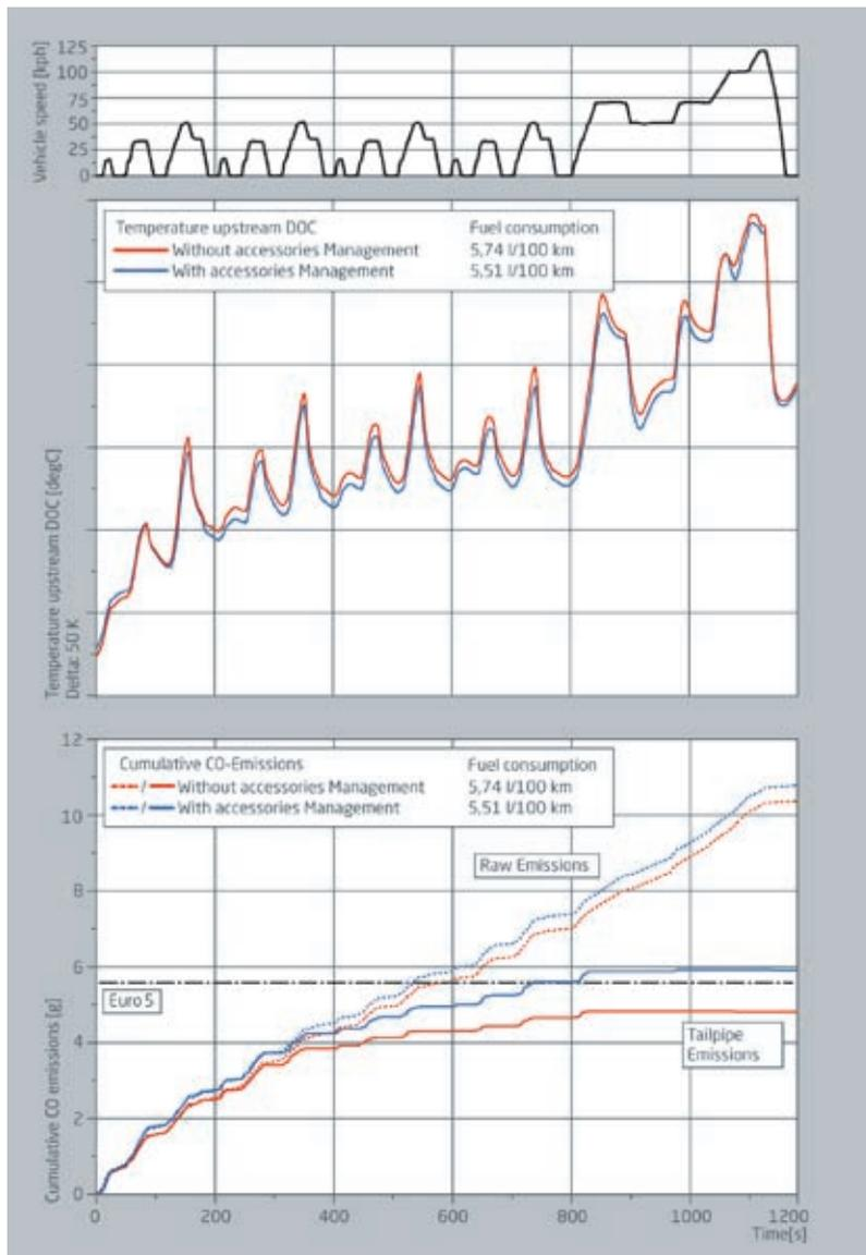
**Figure 2:** Influence of auxiliaries management on CO emissions and exhaust-gas temperature upstream of the DOC
