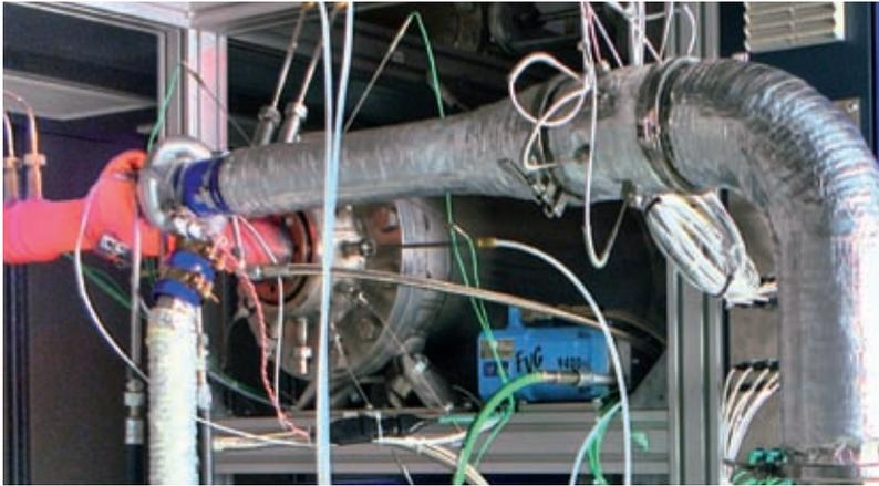
Figure 1: Measurement pipes; V-Clamp quick-connectors
