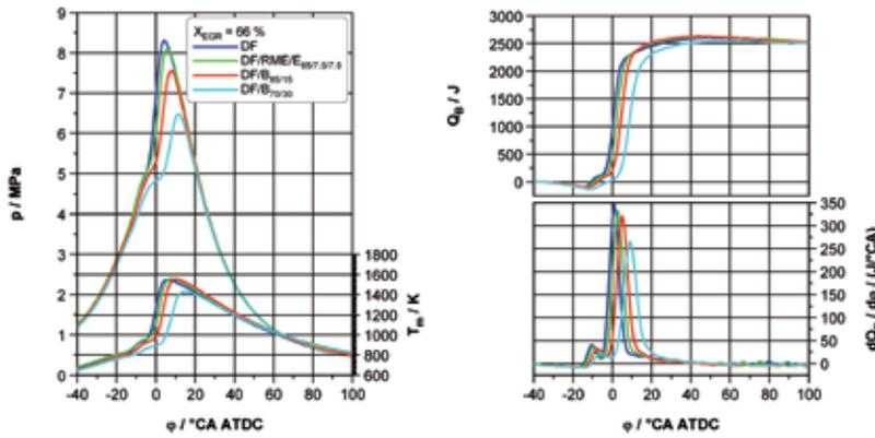
Figure 6: Combustion pressure p and heat release data QB, EGR rate of 66 % for different fuels at HDC, IMEP = 600 kPa
