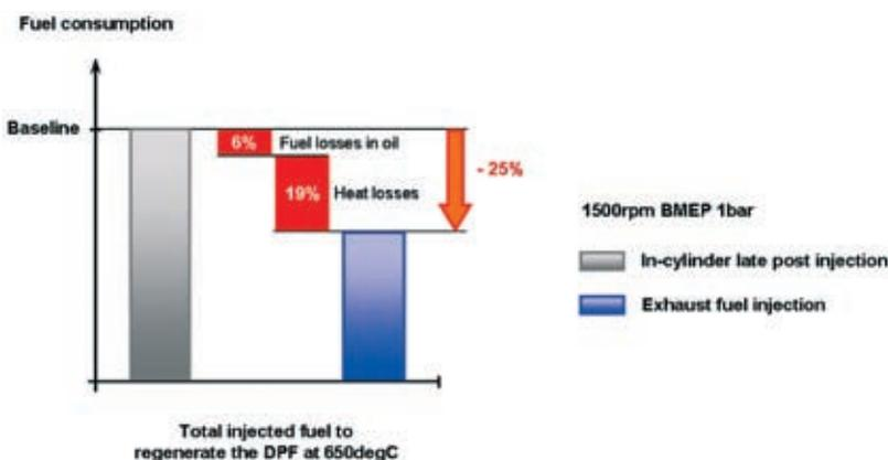
Figure 10: Comparison of the total fuel injected when using exhaust fuel injection versus late post-injection to regenerate the DPF at 1500 rpm / B<sub>MEP</sub> 1bar
