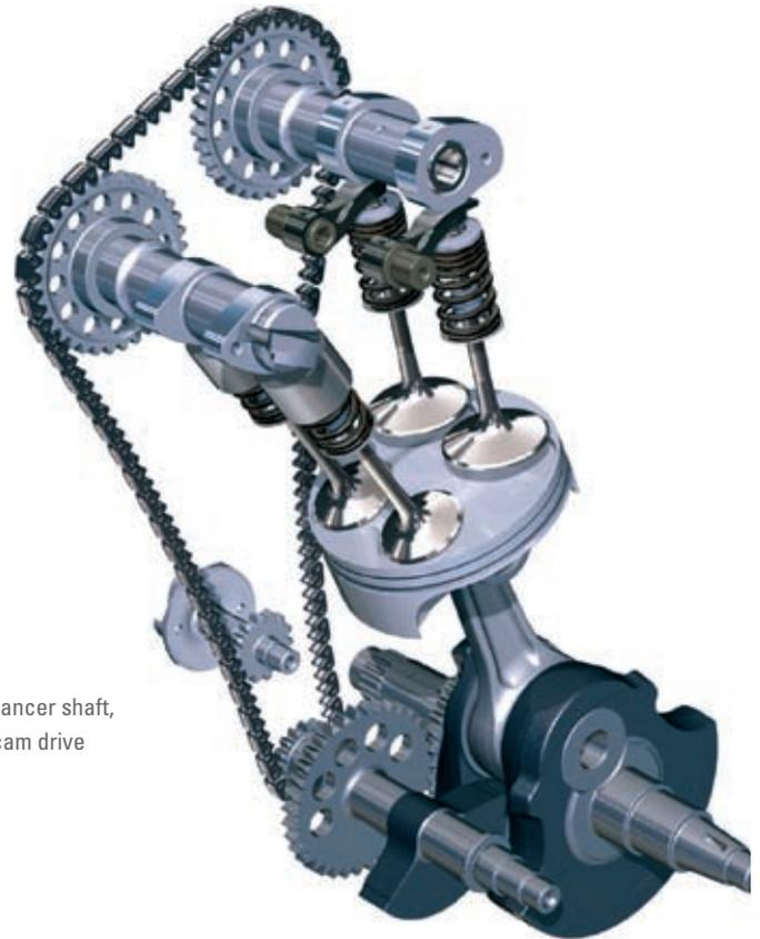
**Figure 5:** Balancer shaft, valve train, cam drive
