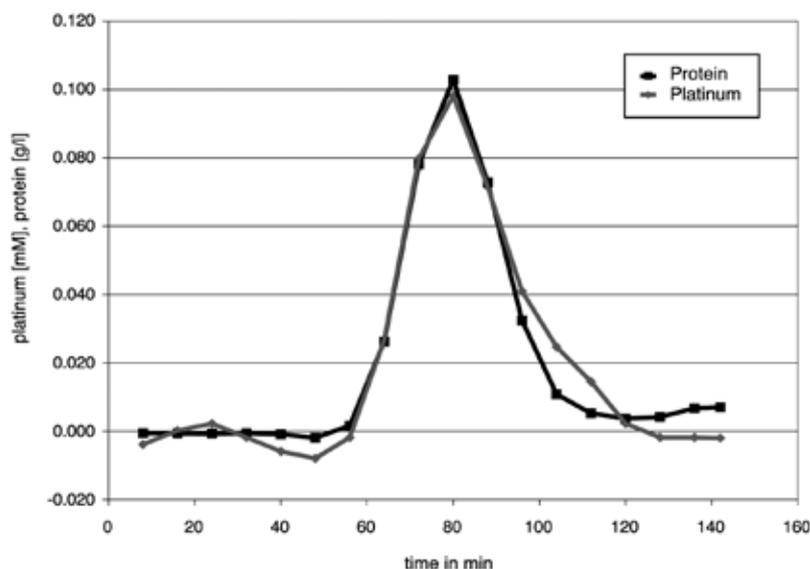
**Figure 2:** Retention diagram of a Platinum-Biotemplate solution – the accordance of time of maximum concentrations at the column outlet gives indications between both components
