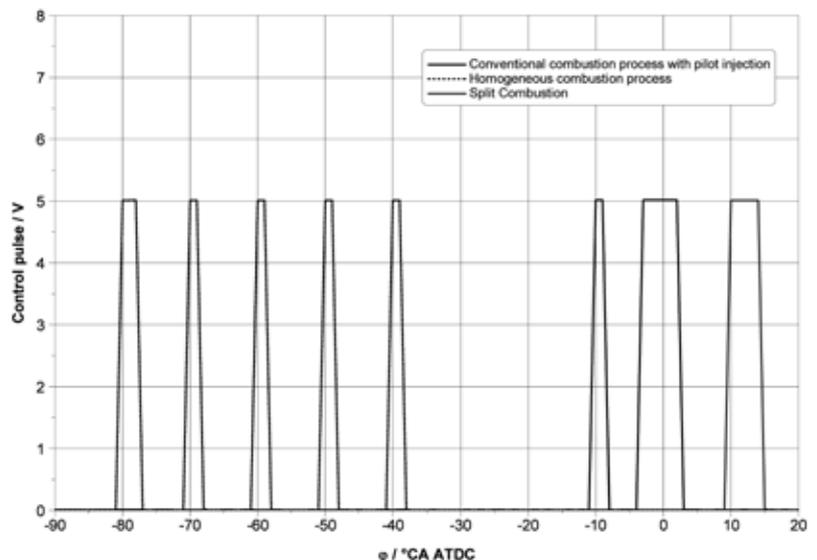
**Figure 3:** Injection patterns for the three combustion processes
