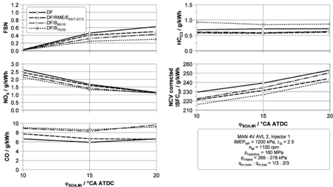
Figure 7: Emissions and consumption at split combustion, IMEP = 1200 kPa
