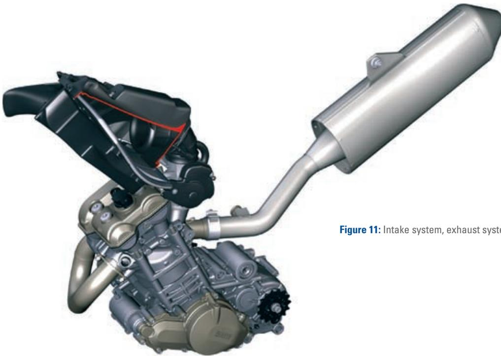
Figure 11: Intake system, exhaust system
