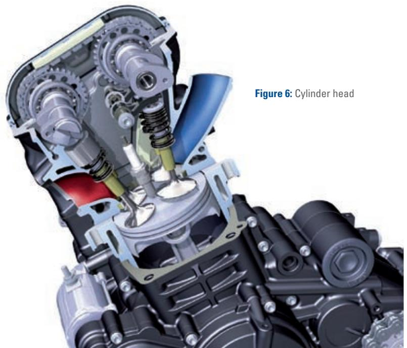
**Figure 6:** Cylinder head
