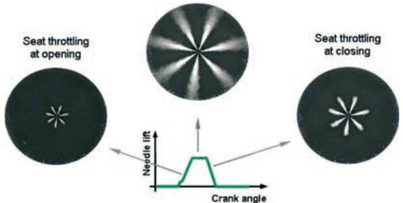
**Figure 6:** Visualization of the seat throttling effect on the fuel sprays during nozzle opening and closing
