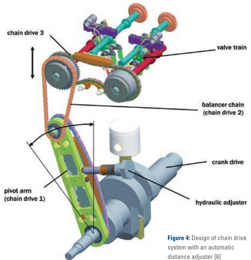
**Figure 4:** Design of chain drive system with an automatic distance adjuster [6]
