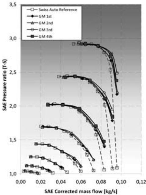
**Figure 8:** Good correlation example of repeated runs for the pressure ratio on Saab/GM and Swissauto test rigs
