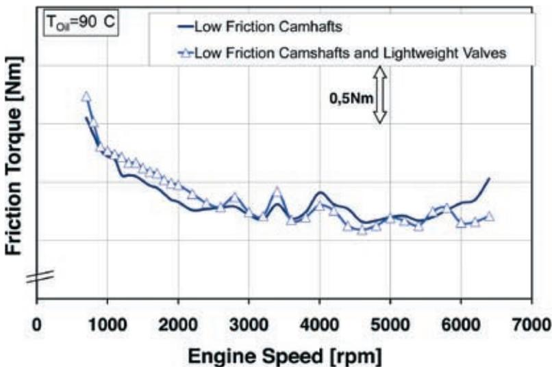
Figure 4: Comparison of Low Friction Camshafts with standard valves and lightweight valves with reduced valve spring forces
