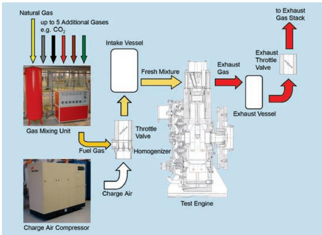
**Figure 2:** Schematic of the test assembly’s set-up
