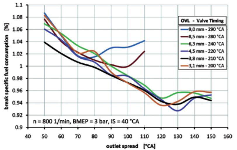
Figure 10: BSFC over exhaust spread with throttle-free load control
