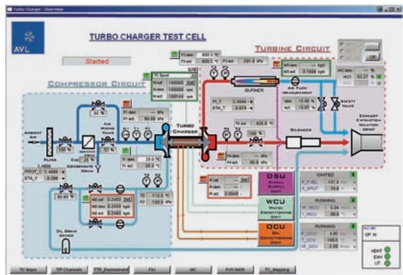
Figure 2: AVL Puma Open – turbocharger application GUI
