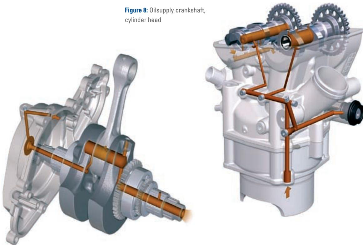
A riser line in the cylinder and cylinder head supplies the chain tensioner and camshaft bearing with oil, Figure 8. From the camshaft plain bearing points, the floating pairs of cam followers and barrel tappets are specifically lubricated by means of an intermittent oil supply.
