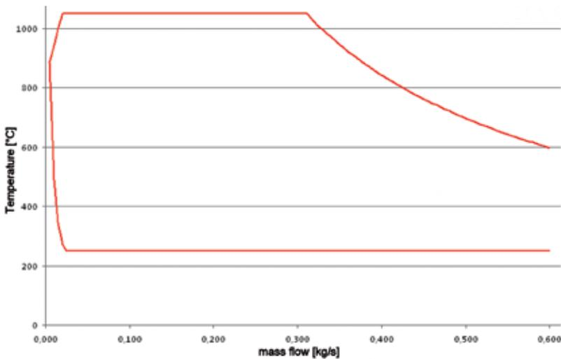
Figure 5: Diesel burner; temperature versus mass flow chart
