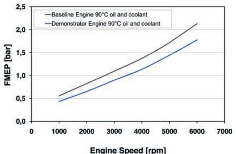
Figure 7: Engine friction – comparison between baseline engine and demonstrator engine
