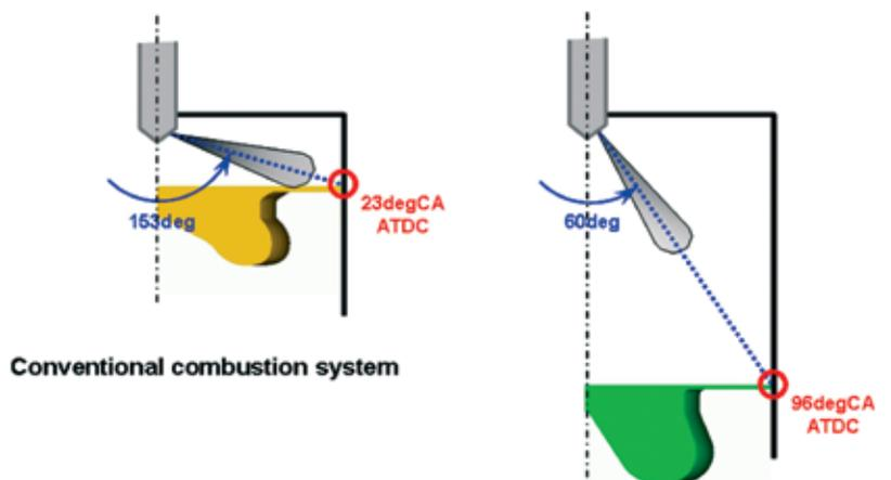
**Figure 7:** Spray design (nozzle tip protusion and cone spray angle) of the conventional and new combustion systems
