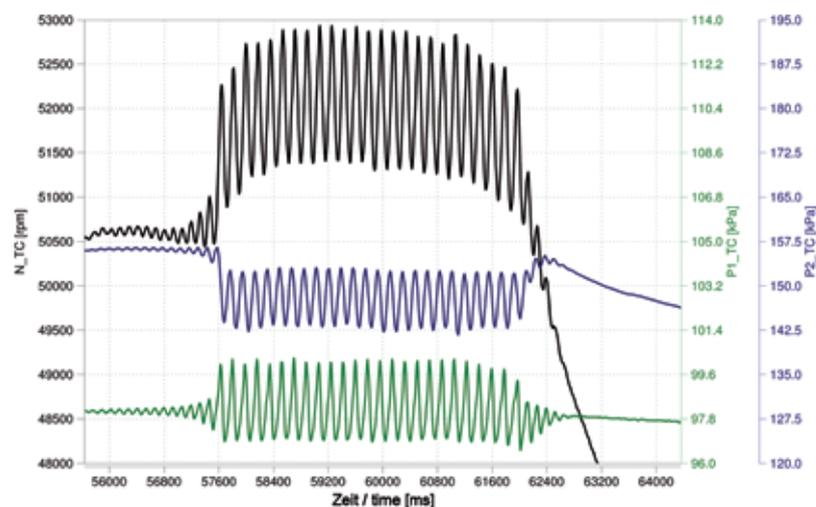
Figure 7: Sensor reading example during surge
