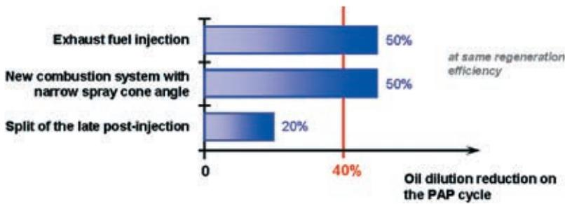
**Figure 11:** Comparison of the different solutions in terms of oil dilution reduction on the PAP cycle in comparison to the standard in-cylinder strategy (up to two late post-injections)
