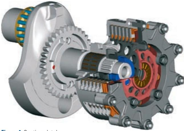
**Figure 4:** Section clutch
