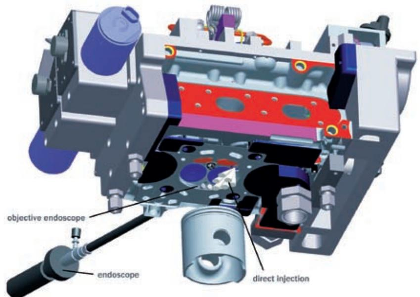
**Figure 5:** Integration of optical measurement technology and direct injection
