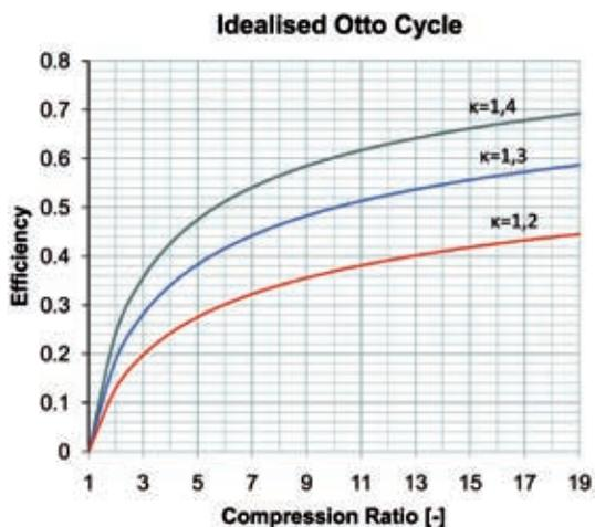
**Figure 1:** Thermal efficiency of idealized otto cycle with different compression ratios
