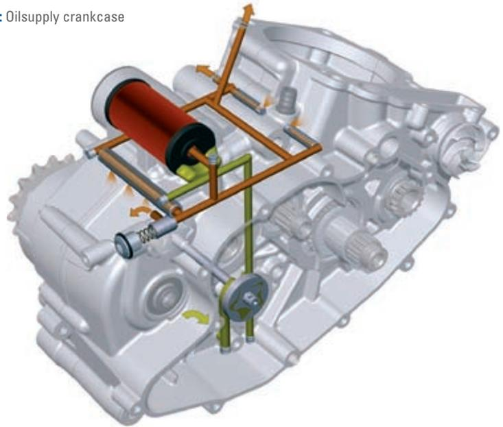
In order to supply pressure oil to the engine, the smaller of the two pumps draws the engine oil through a screen from the oil sump on the transmission side, Figure 7. Next the pressure oil is passed through the filter element and then applied to the main oil duct with the spring-
