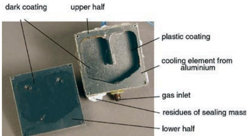
**Figure 1:** Contaminated micro gas cooler
