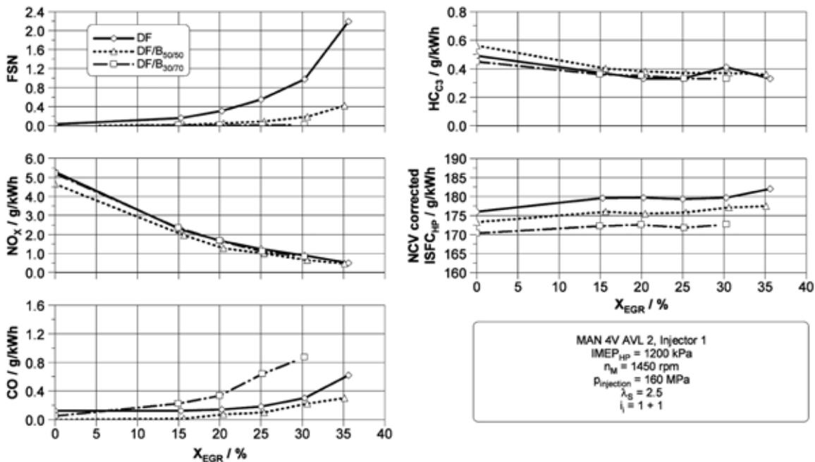
**Figure 10:** Emissions and consumption at conventional combustion process
