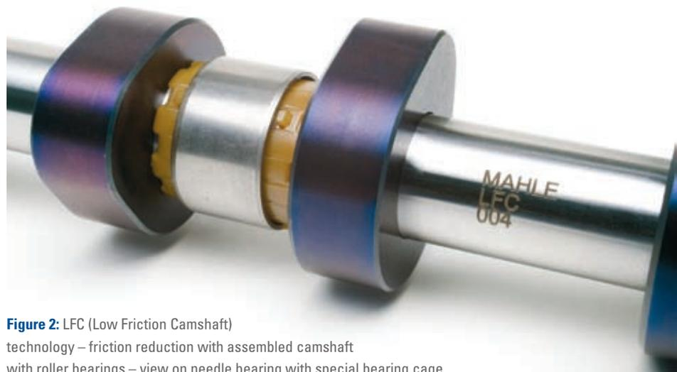
**Figure 2:** LFC (Low Friction Camshaft) technology – friction reduction with assembled camshaft with roller bearings – view on needle bearing with special bearing cage
