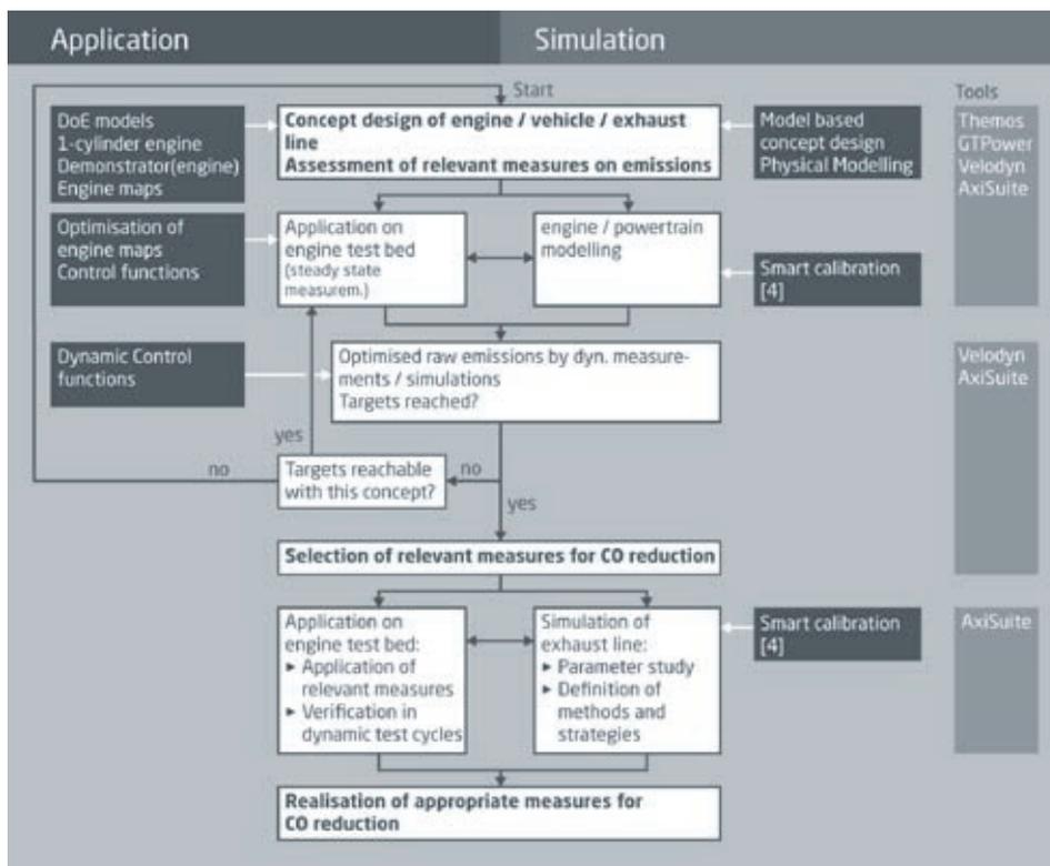
**Figure 6:** Interaction of calibration and simulation in IAV's development process
