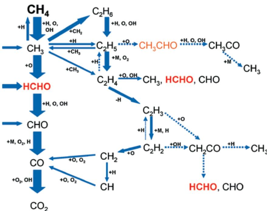
Figure 1: Reaction scheme for the combustion of methane [4]
