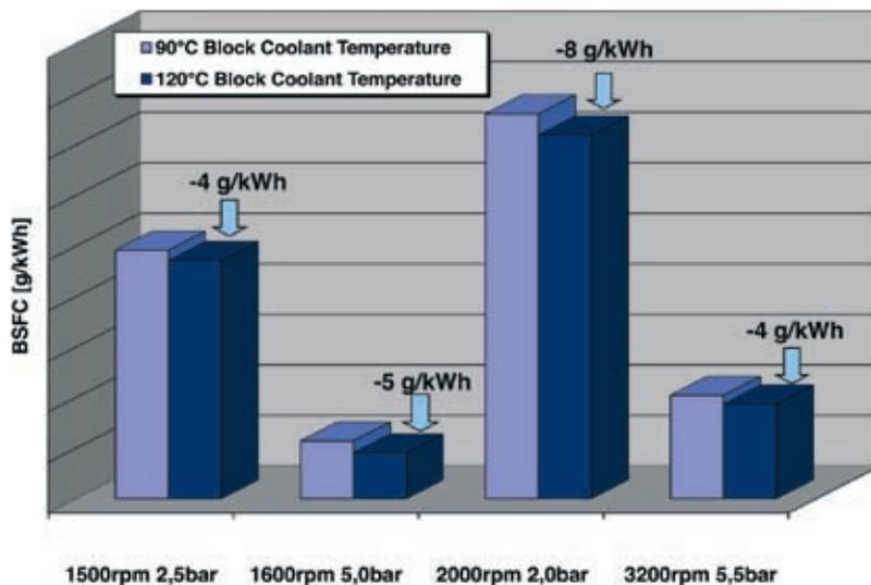
Figure 6: Fuel consumption results with split cooling system
