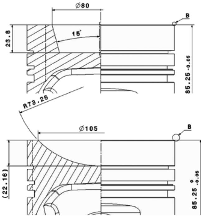
**Figure 11:** Geometry of the original piston (top) and the piston with spherical shaped piston recess (bottom)
