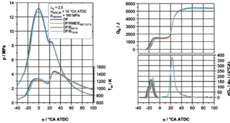
**Figure 8:** Heat release at split combustion with  $\phi_{SOA,MI} = 10^\circ$  CA after TDC for different fuels, IMEP = 1200 kPa
