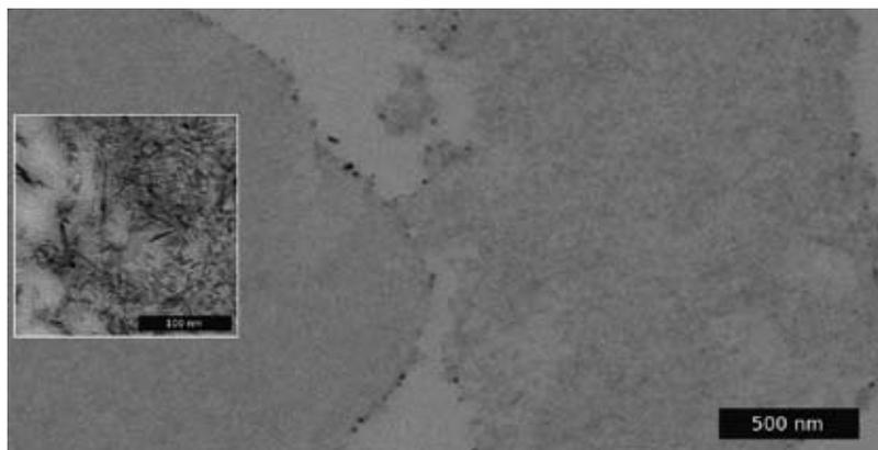
**Figure 3:** Gamma aluminum oxide particles with platinum clusters, TEM micrograph of a micro section
