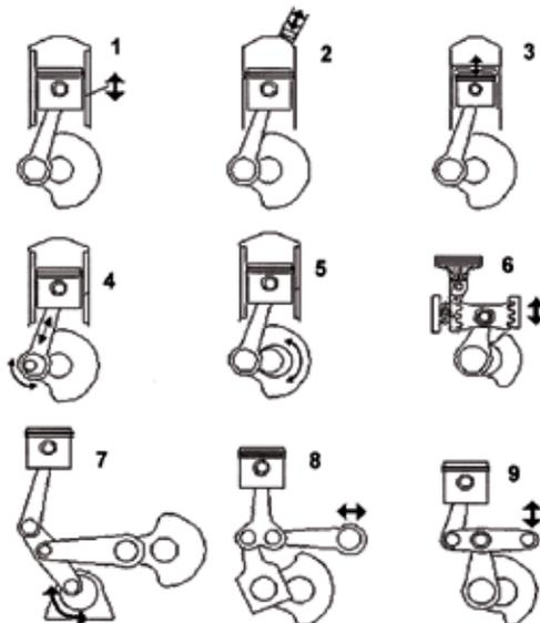
**Figure 3:** Possible designs of variable compression ratio [4]
