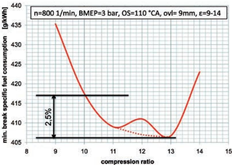
Figure 7: Break specific fuel consumption over geometrical compression ratio (BSFC)
