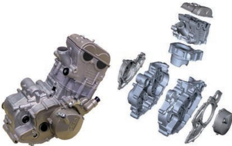
Figure 2: Core engine, engine main parts
