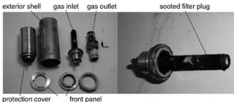
Figure 4: Soot loading of a ceramic filter cartridge before heating
