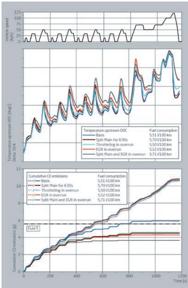
Figure 5: Calibration-based measures for reducing CO tailpipe emissions
