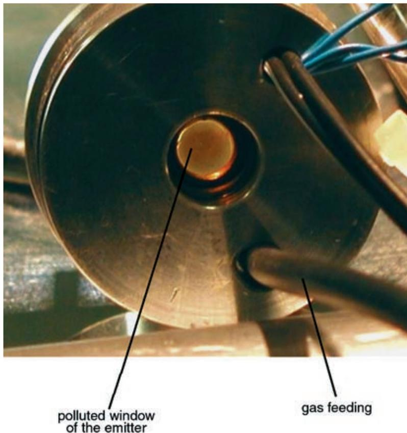
Figure 2: Contaminated emitter window
