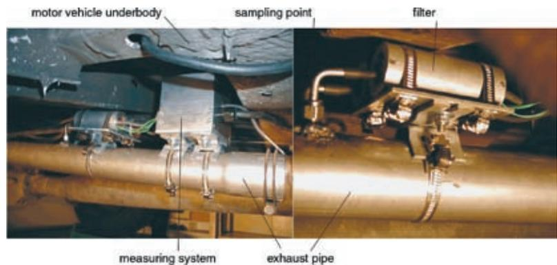
Figure 3: Installation of a regenerative filter
