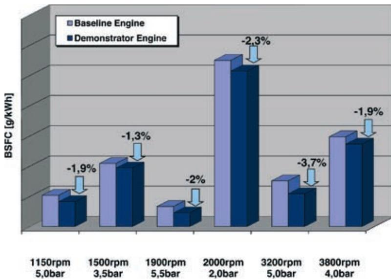
Figure 8: Fuel consumption results of stationary measurements
