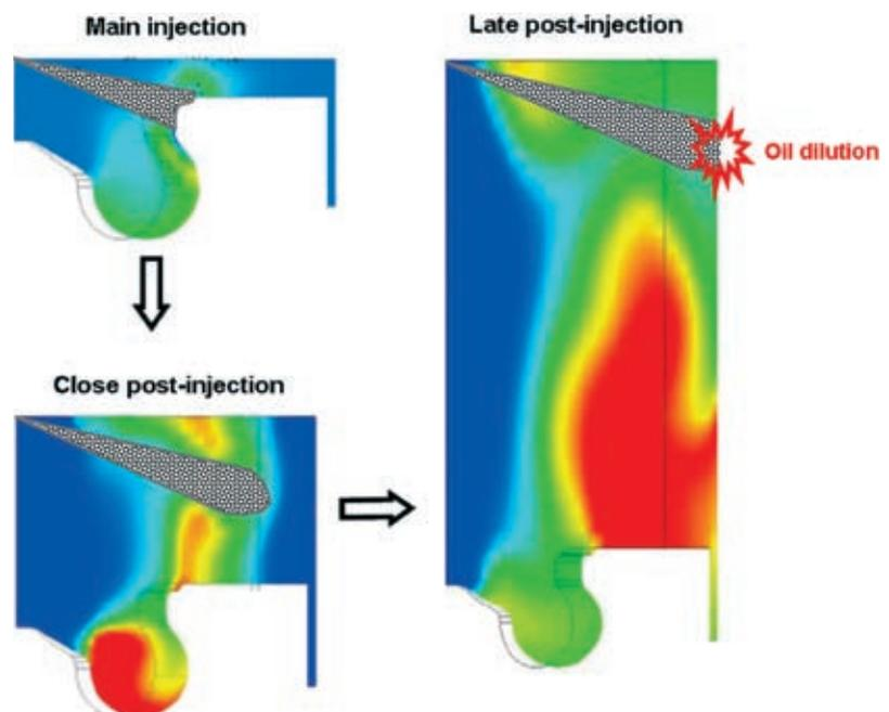
**Figure 4:** 3D CFD showing the temperature gradients and the fuel spray penetration within the combustion chamber at the main, close and late post-injections timings
