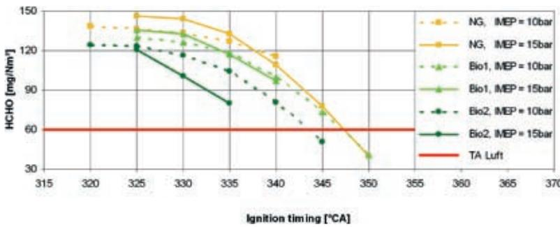
Figure 4: Emissions of formaldehyde for variation of fuel gases at AVL520LVK
