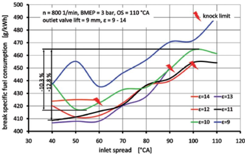
Figure 6: Break specific fuel consumption (BSFC) over IS at different geometrical compression ratios
