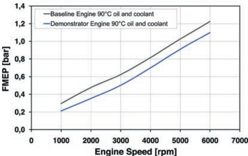
Figure 5: Comparison engine block friction of baseline engine and demonstrator engine
