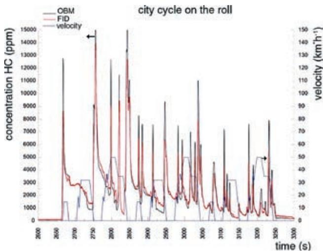
**Figure 5:** Comparison of the hydrocarbon concentrations with certified large analysers and with the OBM system
