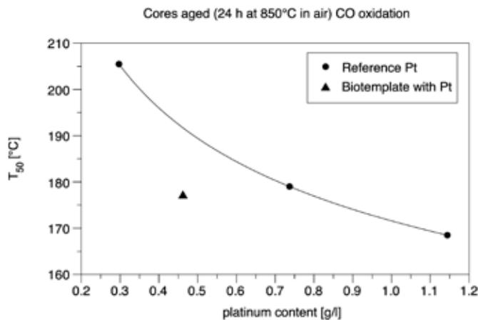
**Figure 4:** Comparison of light-off-temperatures of an impregnated core using biotemplates with reference samples without biotemplates
