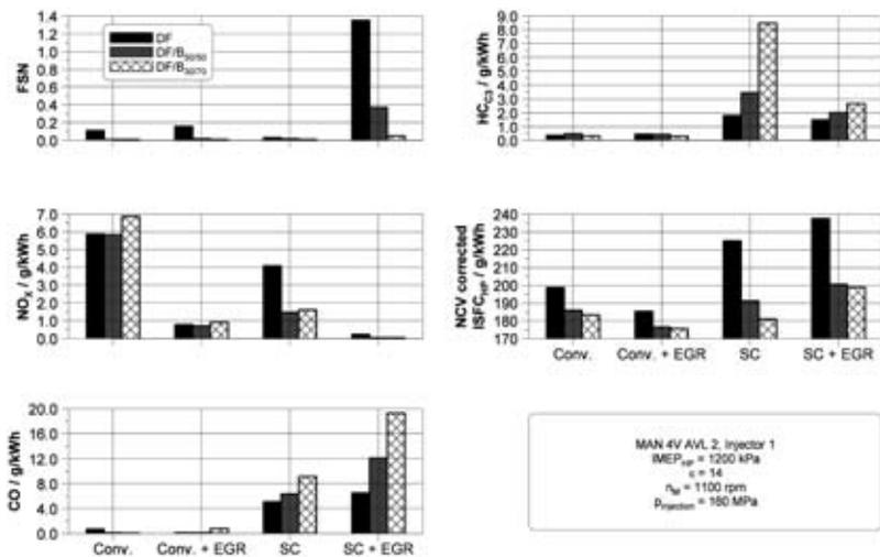
**Figure 9:** Emissions and consumption for different blends and combustion processes
